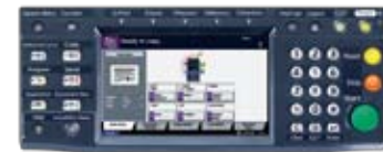
The full-colour, wide-screen touch-panel provides fast access to all functions.
